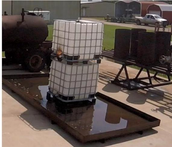
*Figure 3.7: Second Tier IBC Set-up*
