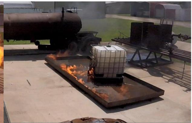
Figure 3.6: Pool fires and burning IBC following flare-up
