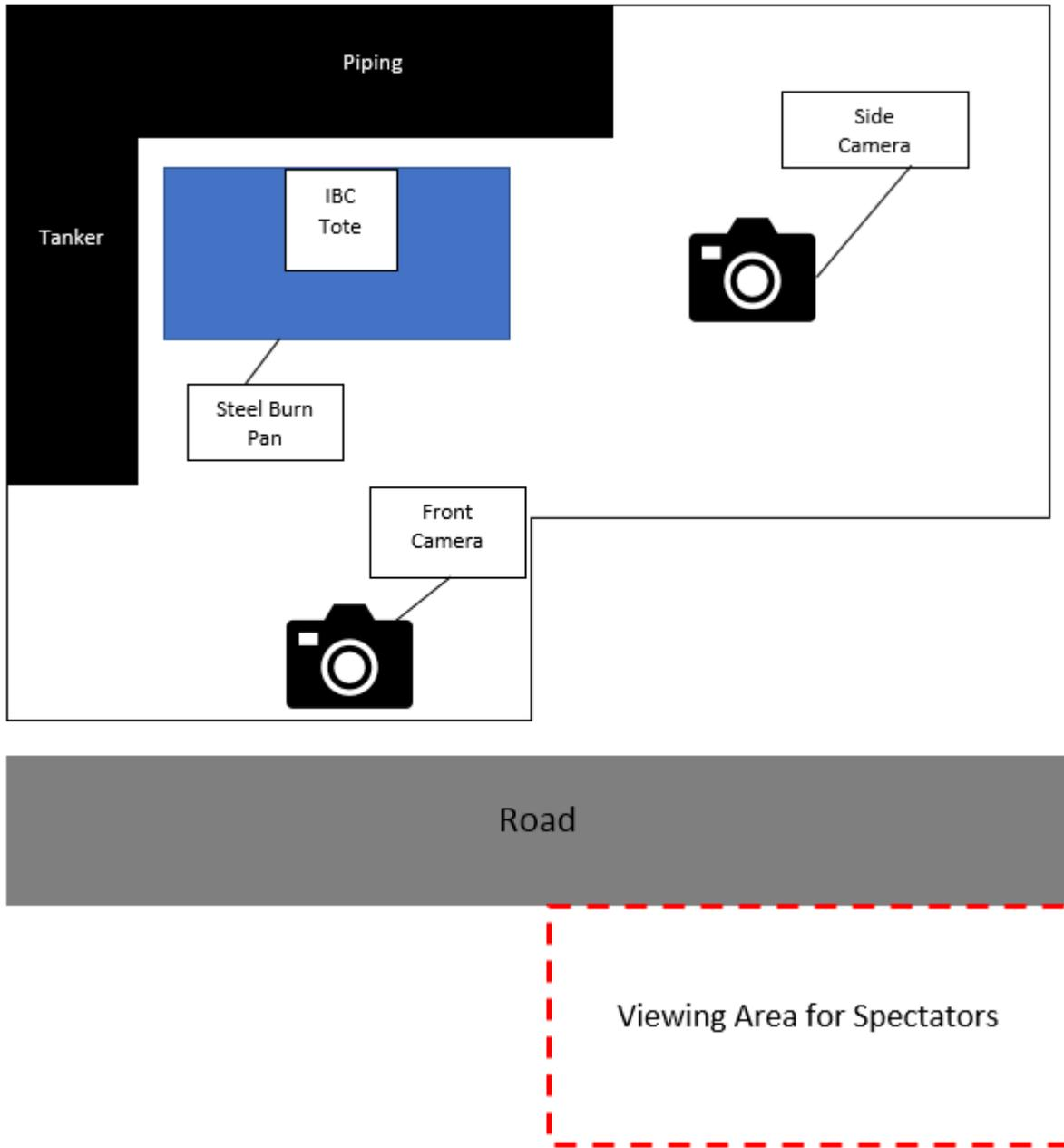
Figure 2.1: Bird's Eye View of Test Layout
