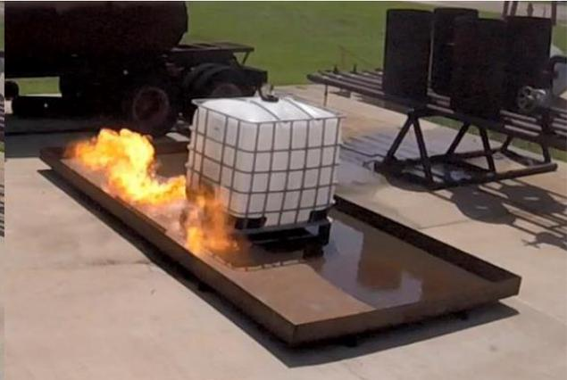
Figure 3.4: Initial vapor ignition
