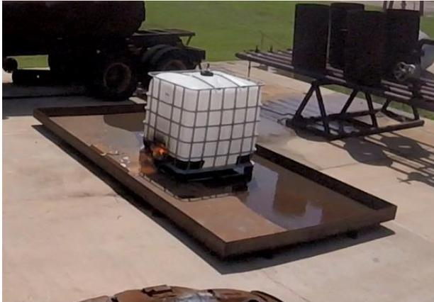
Figure 3.3: IBC inflation and initial vapor release
