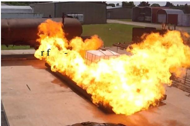
Figure 3.5: Fully ignited vapor cloud
